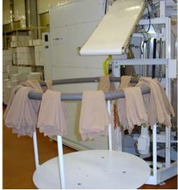
Stockings or pantyhose are stacked on a storing circle with a capacity of 14 stacks.
